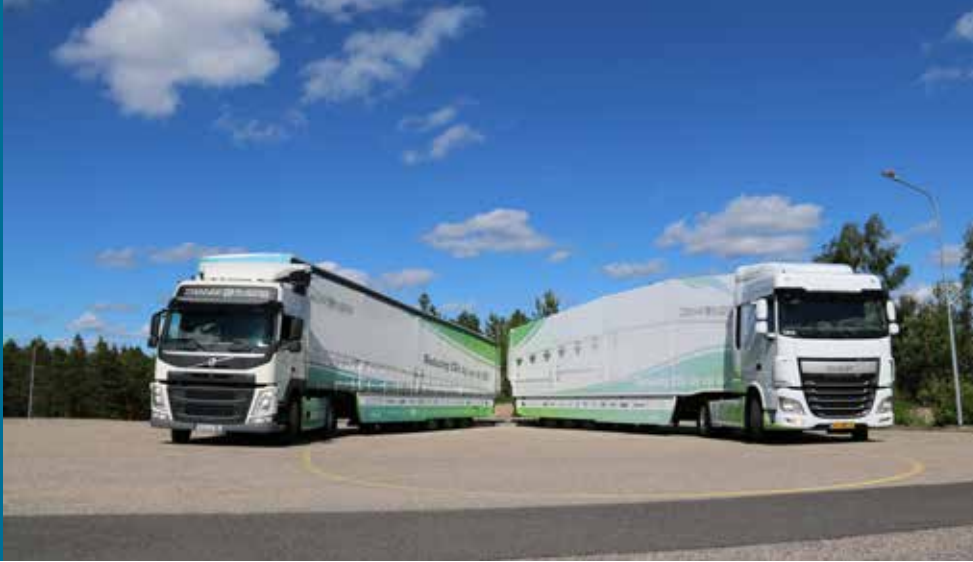
Realized TRANSFORMERS trucks Hybrid-on-demand trailer (left), Load-optimization trailer. (right) © www.transformers-project.eu
