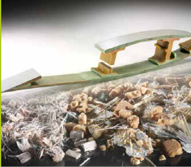
Composite rotor blade: cross section (above) and shredded (below).
