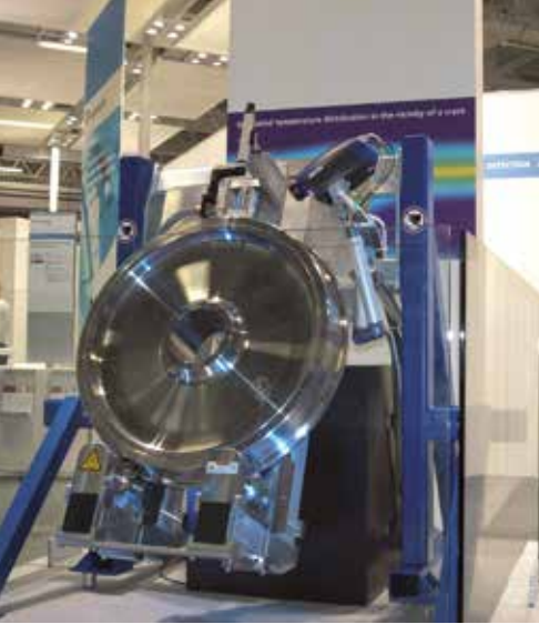
Demonstrator for active thermography on rail wheels.
