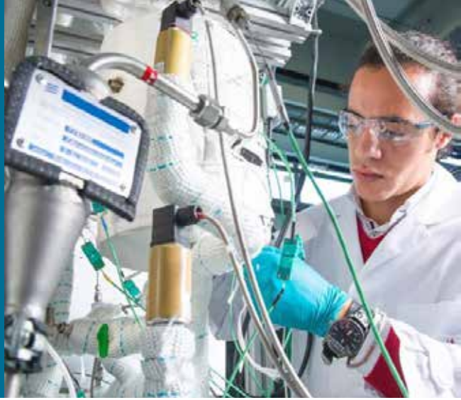
Fraunhofer ISE mini-plant for methanol production from CO 2 and H 2 . © Fraunhofer ISE
