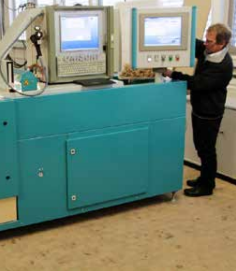
Figure 1: NIR sorting facility for the determination of organic wood preservatives.
