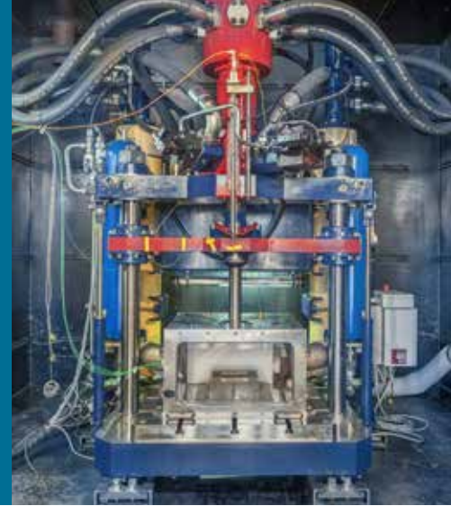
Battery test bench for dynamic tests of loaded cells. © Fraunhofer EMI
