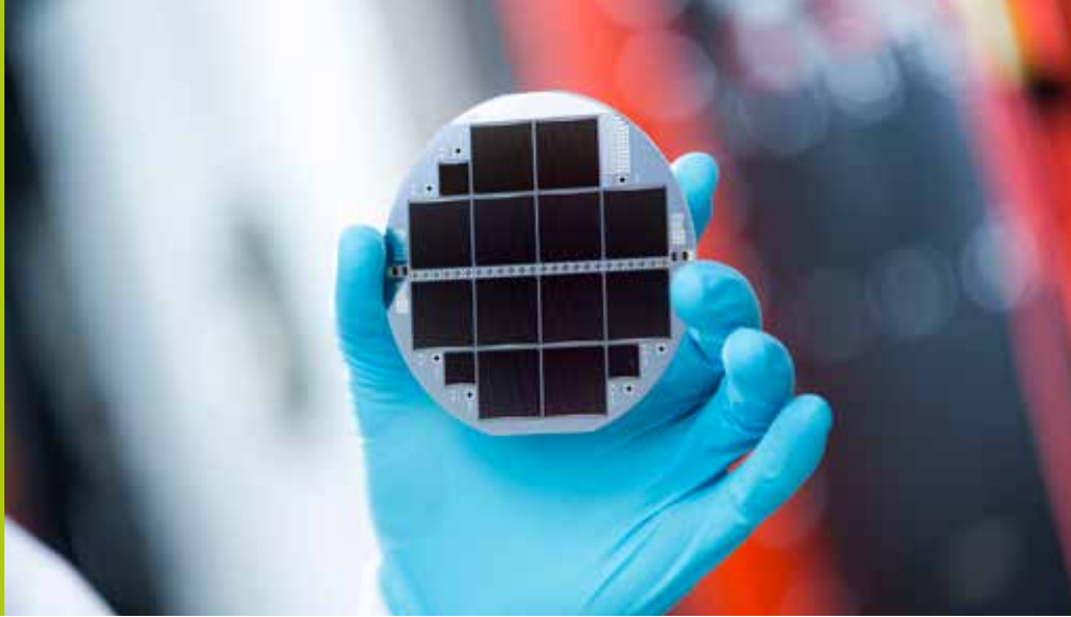
Multi-junction solar cell made of III-V semiconductors and silicon. The record cell converts 33.3 percent of the incident sunlight into electricity. © Fraunhofer ISE/Dirk Mahler
