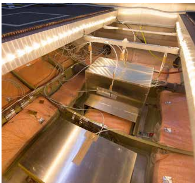
The underfloor area of the cabin demonstrator provides various options to perform thermal tests, using so-called equipment simulators.
