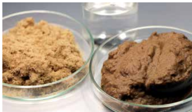
The starting materials for the wood foam: Wood fibers and water are ground to a suspension and foamed. © Fraunhofer WKI
