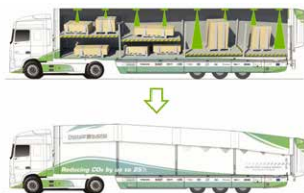
Determination of the load height (above) and adjustment of the roof height (below) image: Fraunhofer LBF
