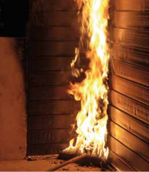
Façade profiles during the SBI test. © Fraunhofer WKI / A. Schirp
