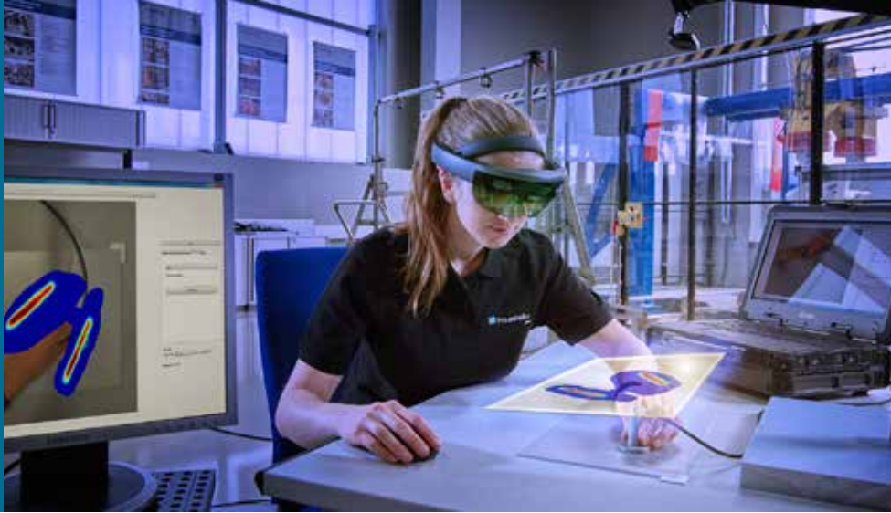
Ready for nondestructive testing with »3D SmartInspect«: An augmented reality system for manual testing of complex components or large surfaces. © Fraunhofer IZFP
