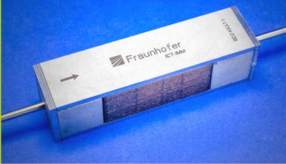
Reactor for biodiesel synthesis under supercritical reaction conditions.
