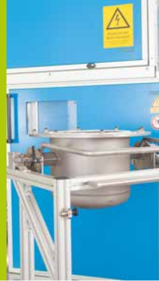
Electro hydraulic fragmentation device at IWKS: phase selective separation of recycling goods. © ImpulsTec GmbH
