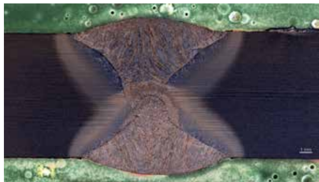
Optical microscope image of the weld structure of a welded joint.
