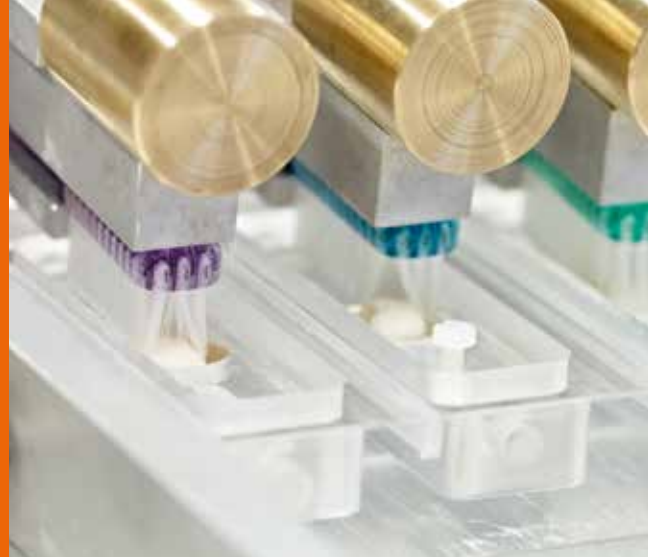
A brushing machine is used to investigate the mechanical impact of dental cleansers on teeth.
