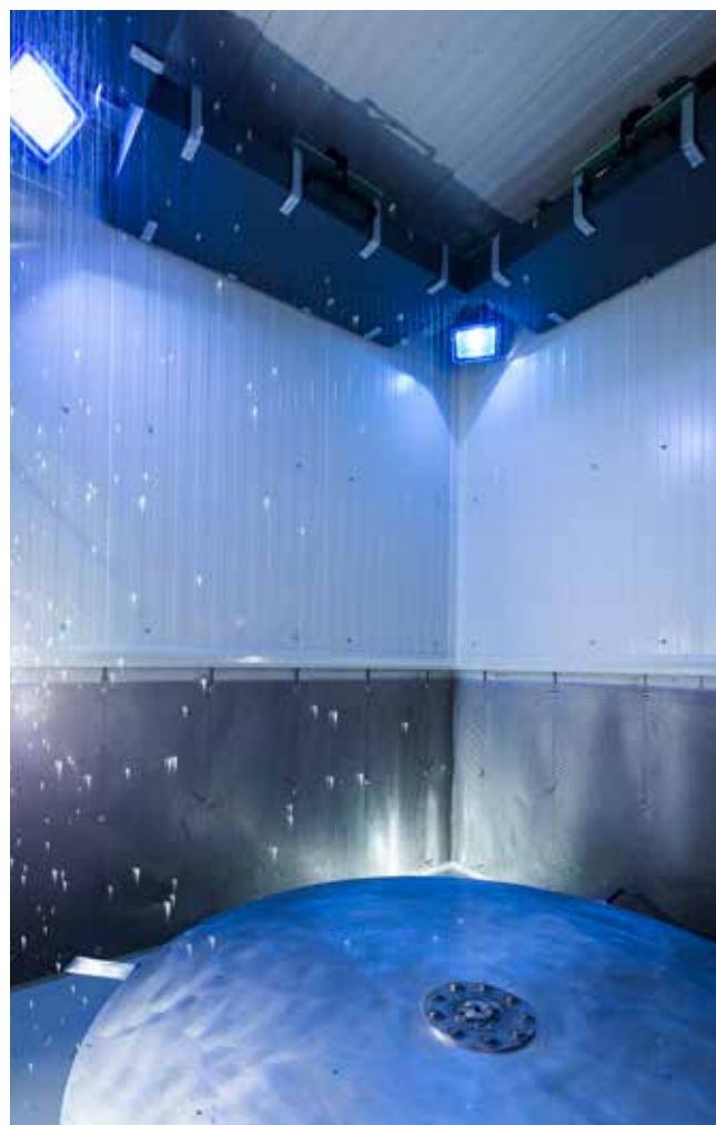
Equipment: Max. speed: 550 km/h, Temperatures: 4°C to 40°C, Variable drop size: 1.5 to 5.5 mm © Jan Meier
